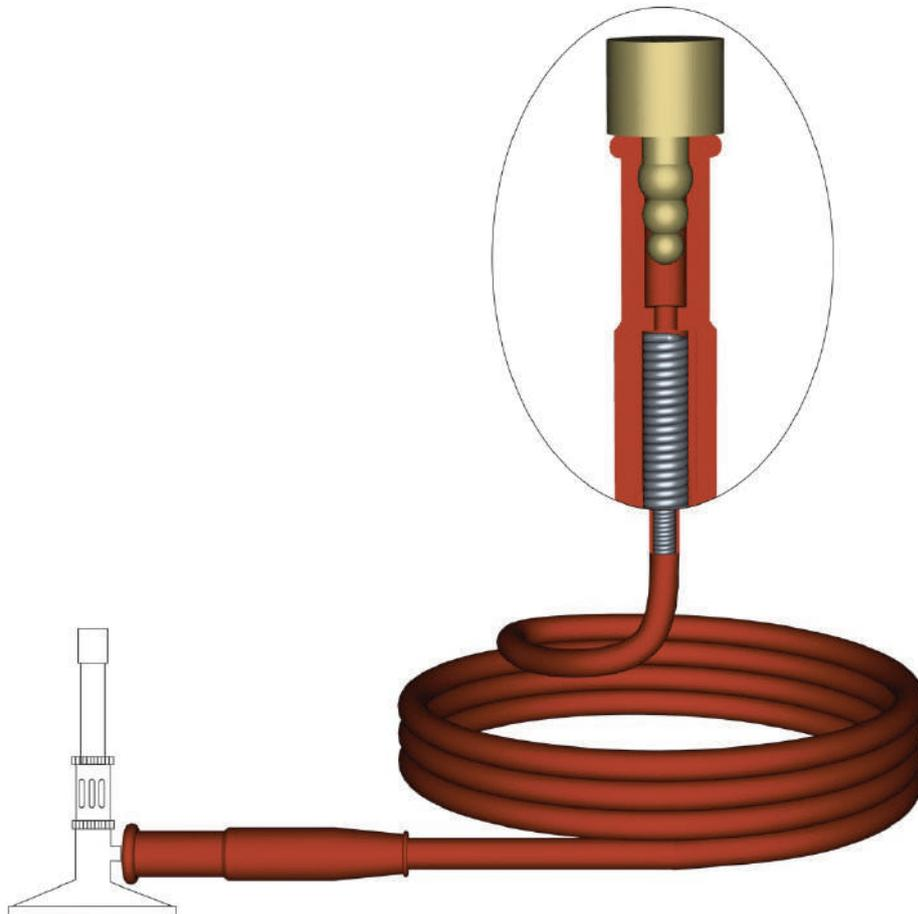
**- Safety flexible gas tube -****Tested and supervised by DVGW (German Association of the Gas and Water Fields) DVGW Test mark****Safety and quality**
